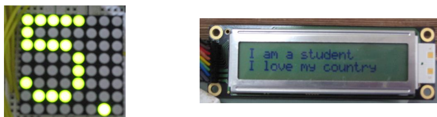
Figure 2: Examples of the results of experiments: (a) 8x8 LED matrix display; (b) LCD display experiment (l-r).
