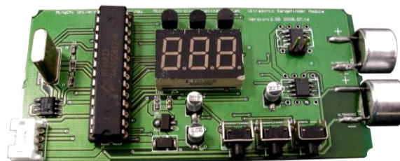
Figure 5: Photograph of the extra-sonic distance measurement system project.
